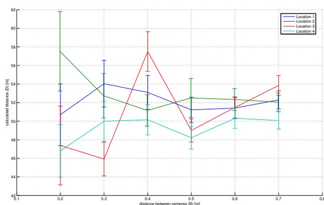
Fig. 165. Calculated distances to marker set at 50m at 4 different locations.
