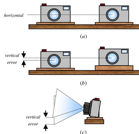
Fig. 1. Proper alignment of the cameras (a) and alignments with vertical errors (b) and (c).
