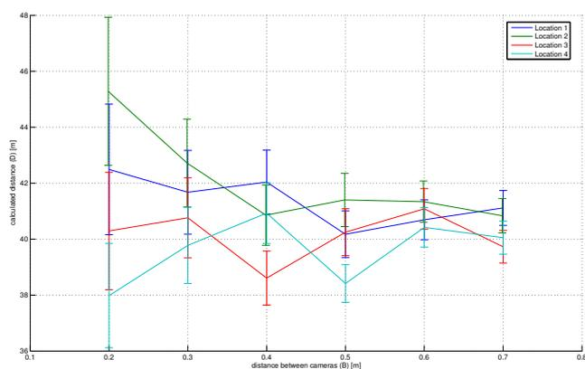
Fig. 15. Calculated distances to marker set at 50m at 4 different locations.
