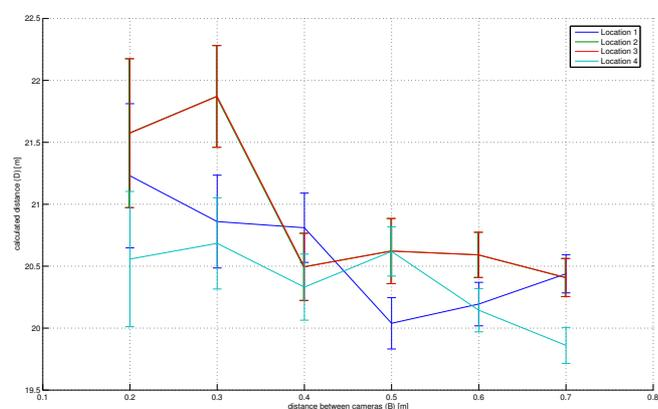
Fig. 13. Calculated distances to marker set at 20m at 4 different locations.
