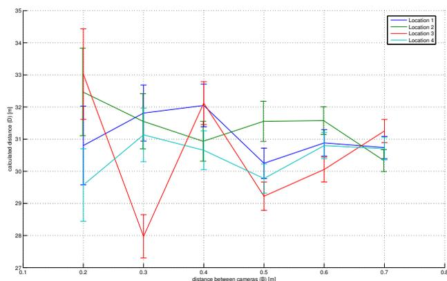
Fig. 14. Calculated distances to marker set at 30m at 4 different locations.
