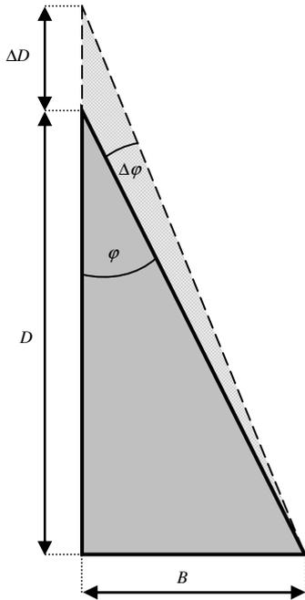
Fig. 5. Distance error caused by 1 pixel positioning error.
