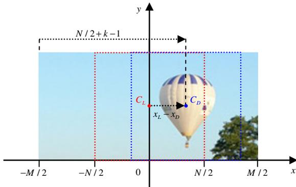
Fig. 9. Calculation of the horizontal distance of the object between left and right picture.
