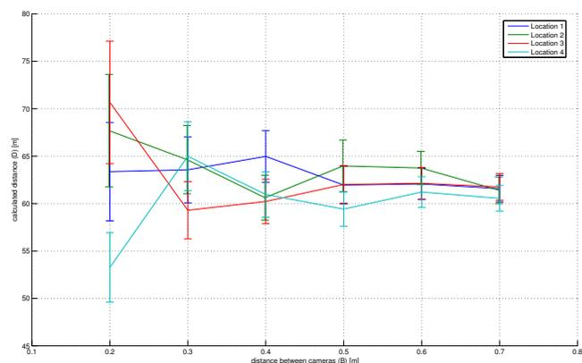
Fig. 176. Calculated distances to marker set at 60m at 4 different locations.
