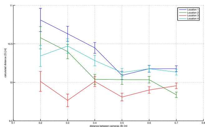
Fig. 12. Calculated distances to marker set at 10m at 4 different locations.
